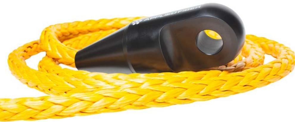
**S**ynthetic ropes for crane applications have already been in development at WireCo for several years. The bright yellow rope, made by Lankhorst Ropes, consists of 12 braided outer strands made of the high-tech material Dyneema. The properties of these special fibres result in a breaking strength equal to a steel rope of the same thick-
