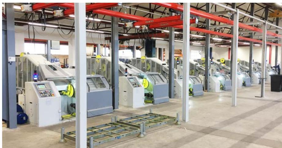
Finally, the coils are transported directly over an additionally constructed access way to the stranding machines in production. This avoids longer storage time and time loss. It also reduces costs and setup times, and optimises material flow. The new spooling centre is then optimally integrated into the supply chain.
