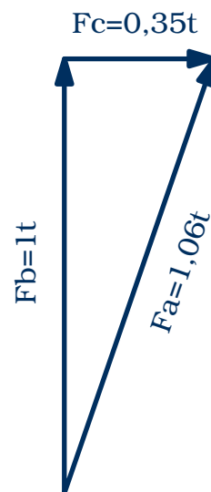
Fig. 5: Force components of the strands
