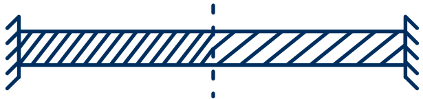
Fig. 30: ...causes lay shortening on the one side (left) and lay lengthening on the other (right).
