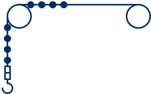
Fig. 45: While lifting the load, half of the twisted rope length passes over the sheave.
