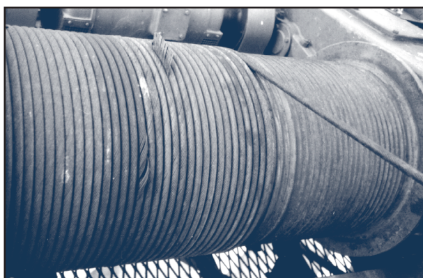
Fig. 49: Birdcaging on the rope drum
