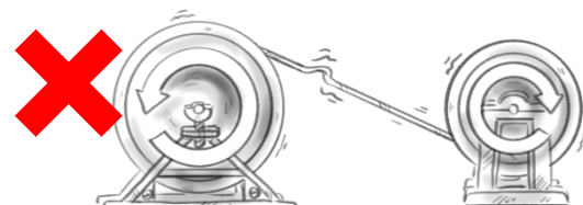
Incorrect winding opposite to bending direction
