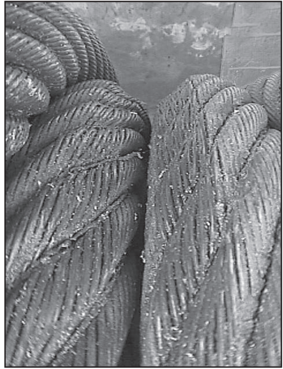
Fig. 26: Consequences of a rope "cutting in"
