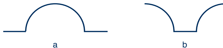
Fig. 3: Definition of one bending cycle
