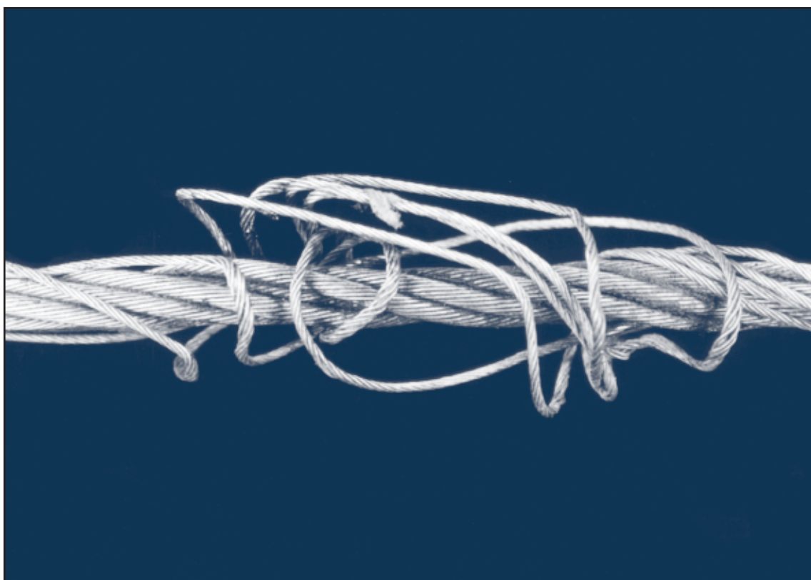
Fig. 38: Surplus length of the inner strands caused by closing the same rope
