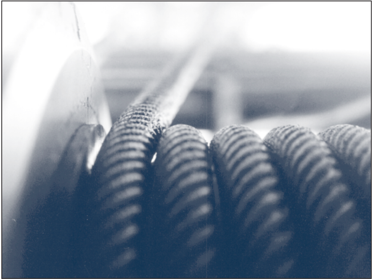
Fig. 44: Under the influence of a fleet angle, the wire rope is pulled against a neighbouring wrap. The outer wires will be damaged at the point of contact.
