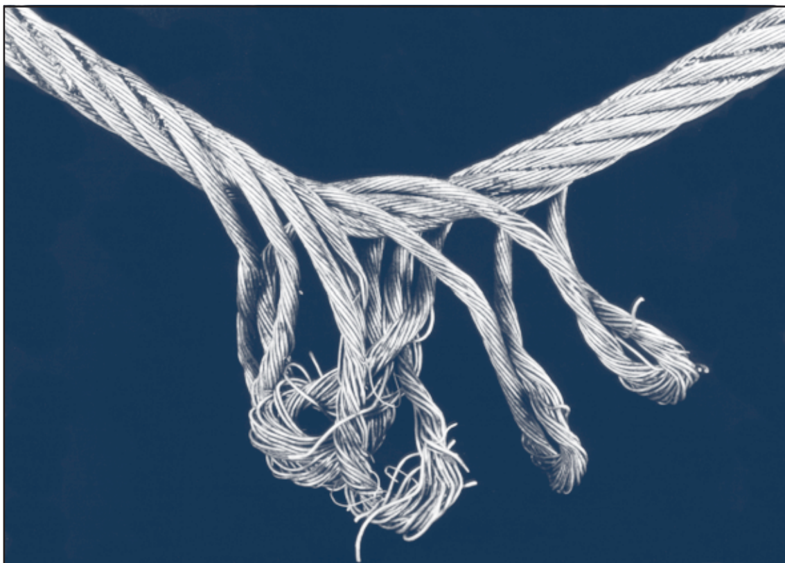
Fig. 37: Surplus length of the outer strands caused by unlaying the rope
