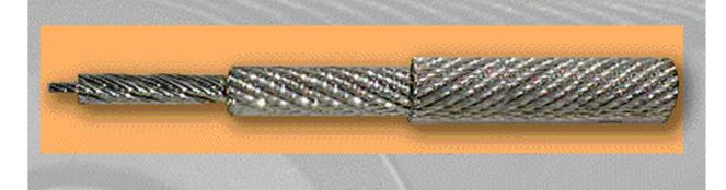
Providing there are no other special conditions that require the use of rotation- resistant ropes, non rotation- resistant ropes should be used in multiple fall conditions.
