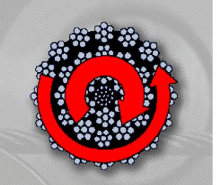
is such that the moments in the core and the outer strands compensate each other over a wide loadspectrum, so that even with great lifting heights no rope twist occurs.
