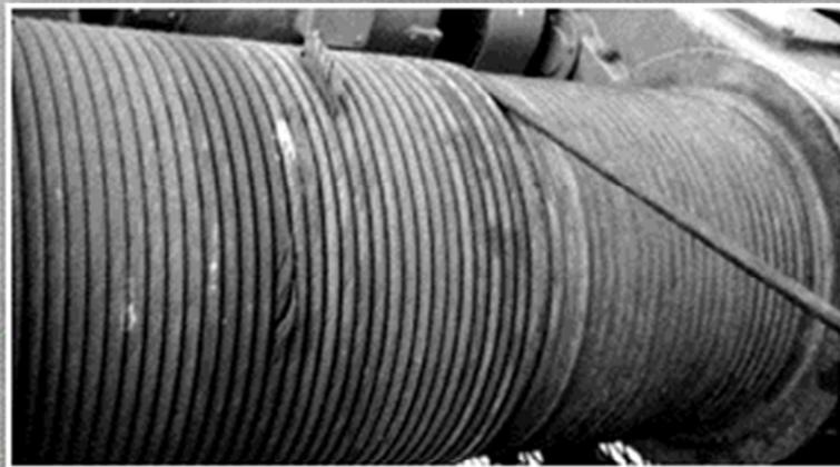
When a twisted rope is unloaded abruptly, a very dangerous situation called 'slack-rope formation' may occur.
