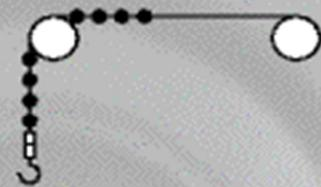
Fig. 42: While lifting the load, half of the twisted rope length passes over the sheave.
