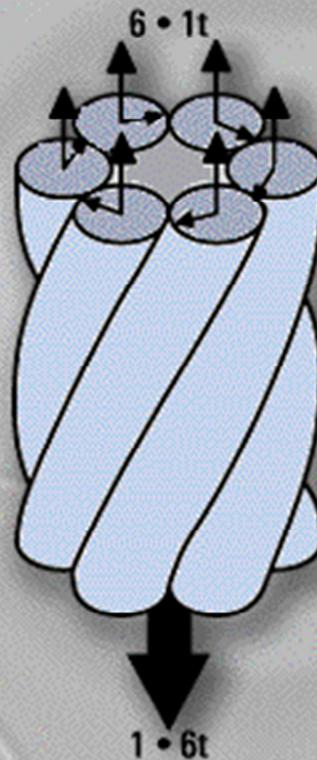
Fig. 3: Closed wire rope
