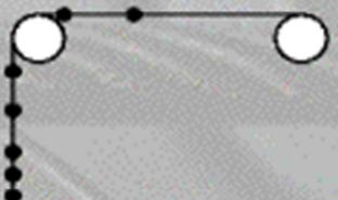
Fig. 44: Part of the twisted rope length runs back over the sheave.
