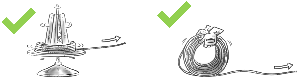
Unwinding with a turntable
