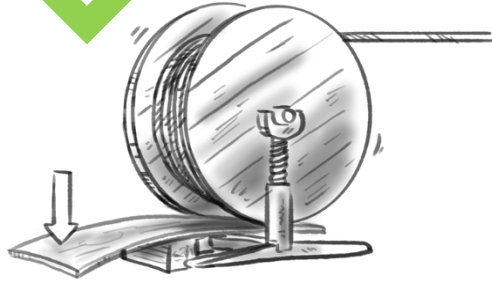
Application of the preload by braking the reel flange
