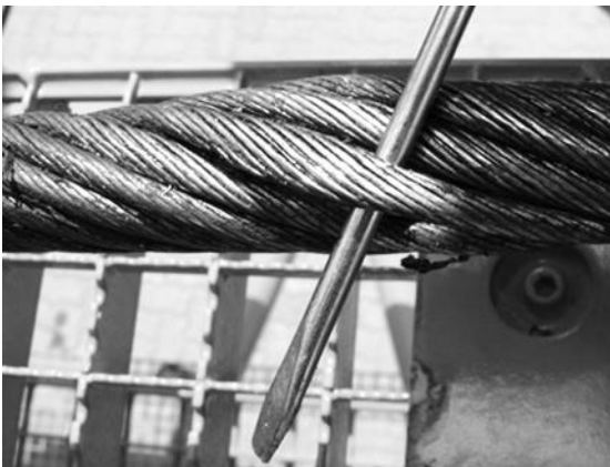
Protruding or deformed core or strand
