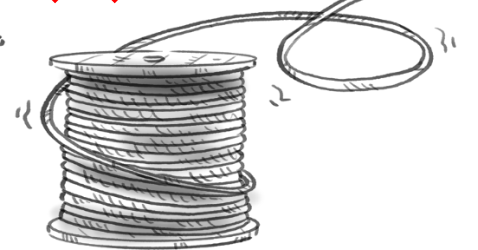
Removal from reel from the side
