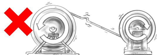
Incorrect winding opposite to bending direction
