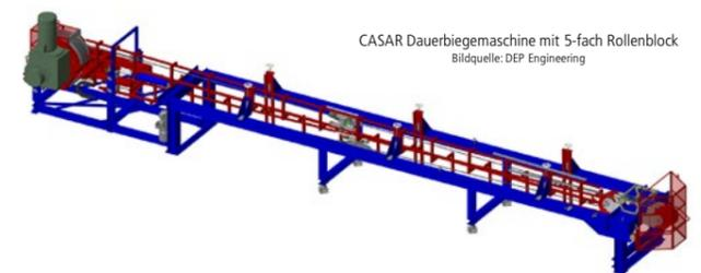
Following diagrams show the service life values determined in the laboratory on a permanent bending machine with the same relative loads and with the same diameter ratio (D / d = 20) for the non-rotation resistant CASAR ropes as well as the rotation resistant CASAR ropes.
