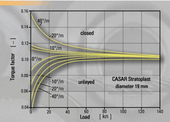
Fig. 28: The changes of the torque factor of a non-rotation-resistant wire rope caused by enforced rotation. The factor k is hardly changed.
