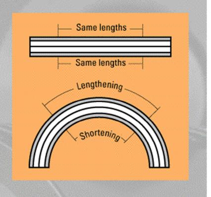
Fig. 2: The change of lengths when bending a bundle of strands
