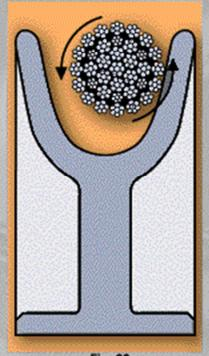
Fig. 30: The wire rope rolls into the bottom of the groove.
