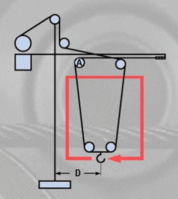
Fig. 48: When lifting and lowering the hook, sheave A does not rotate. Sheave A only rotates if distance D changes
