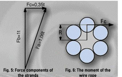
in the strands of the bundle. Even more serious than that is the fact that in each strand a force component Fc is generated in the tangential direction of the rope. In connection with lever arm R to the
