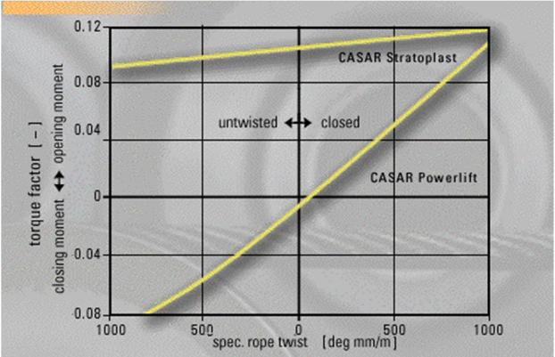
Rotation 2: Torque factors of CASAR Stratoplast and CASAR Powerlift against the rope twist (forcible twist). The high torque of CASAR Powerlift under forcible twist guarantees a high resistance against rotation of the load.
