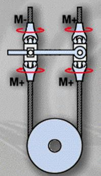
Fig. 57: Connection not secured against rotation between two ropes with different directions of lay
