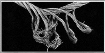
Fig. 36: Surplus length of the outer strands caused by unlaying the rope
