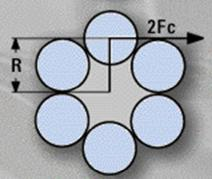
Fig. 8: The influence of the load on the moment of the rope
