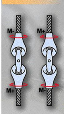
Fig. 54: Correctly connected grab ropes
