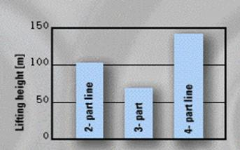
Fig. 20: The influence of the number of parts on the maximum permissible lifting height
