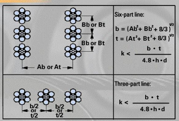
Fig.19b: The calculation of the stability of a block for six- and three-part reeving systems.
