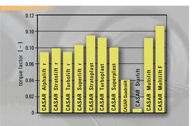
Rotation 1: Torque factors for different CASAR Special Wire Ropes. The torque factor is defined as the moment of the rope under a given load, divided by the load and the rope diameter.
