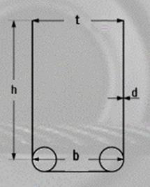
Fig. 18: Dimensioning the reeving
