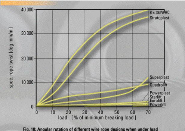
The actual design factor of the reeving system is dangerously reduced by the use of a swivel in combination with these rope constructions.
