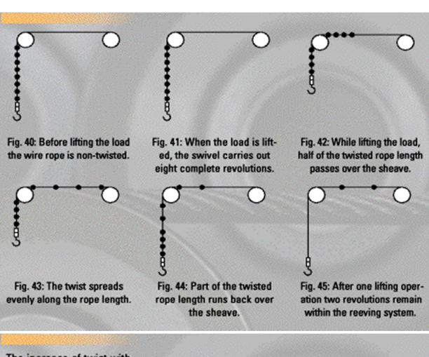
The increase of twist within the system in the course of further lifting operations may lead to different consequences for the rope.
