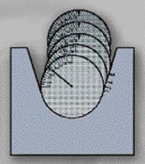
Fig. 32: Great twist of a rope when the fleet angle is 5°
