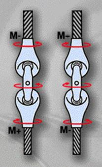
Fig. 56: Connection of wire ropes with equal direction of lay but different diameters
