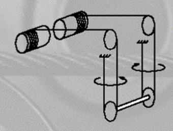
Fig. 22: Crane with left-hand lay and right-hand lay wire ropes
