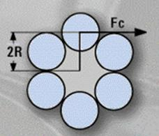
Fig. 7: The influence of the nominal rope diameter on the moment
