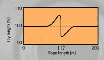
Fig. 33: Change of rope lay length caused by a sheave
