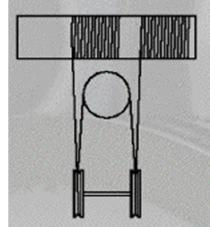
Fig. 23: Crane with two left-hand lay rope drums
