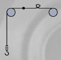
Fig. 47: Formation of a loop when a twisted rope is sagging or slack
