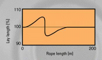
Fig. 35: The change of the lay length caused by a drum with the wrong direction of grooving
