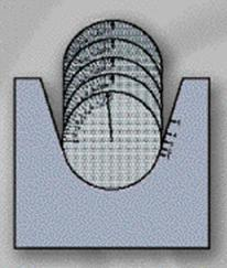
Fig. 31: Slight twist of a rope when the fleet angle is 1°
