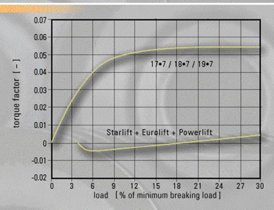
Fig. 13: Torque factor of different wire rope designs in dependence on load
