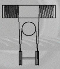
Fig. 24: Crane with one left-hand lay and one right-hand lay drum.
