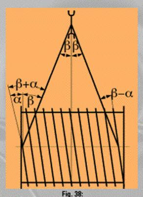
Reducing the angles by increasing the diameter of the drum
