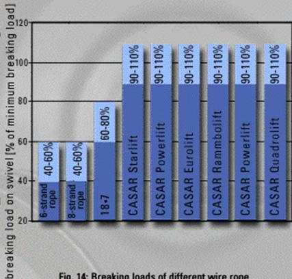
Fig. 14: Breaking loads of different wire rope designs in a break test with an open swivel
