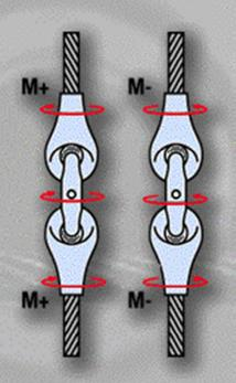
Fig. 55: Incorrect connection of grab ropes. The ropes unlay each other.
