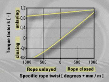
Fig. 25: When, for instance, rotation is enforced by slewing the crane, rotation-resistant ropes develop much greater counteracting moments than non-rotation-resistant ropes.
