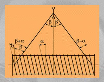
Fig. 34: Fleet angles at the drum and the sheave
