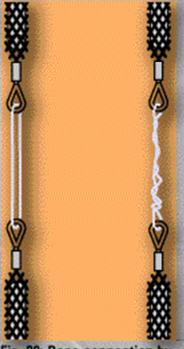
Fig. 39: Rope connection by means of Chinese Fingers. Before (left) and after installation (right).
