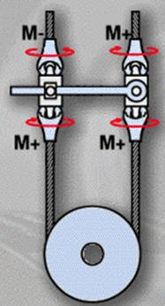
Fig. 58: Connection secured against rotation between two ropes with different directions of lay
