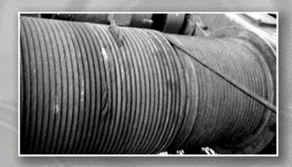
When a twisted rope is unloaded abruptly, a very dangerous situation called 'slack-rope formation' may occur.
