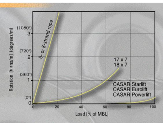
Fig. 15: Angular rotation of different rope constructions in a break test with an open swivel
