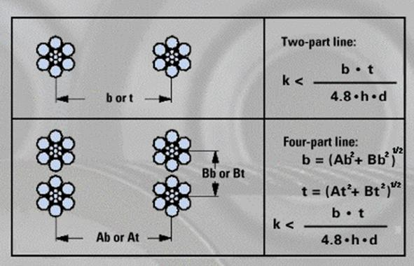
Fig.19a: The calculation of the stability of a block for two- and four-part reeving systems.
