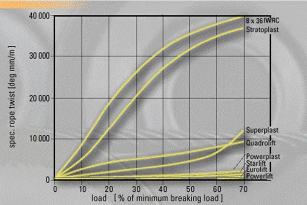
Rotation 3: Specific rope twist as a function of the load. When tested on a swivel, 6-strand and 8-strand ropes untwisted under very low loads. CASAR Powerlift, CASAR Starlift and CASAR Powerplast only started untwisting at high loads.
