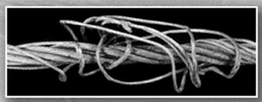
Fig. 37: Surplus length of the inner strands caused by closing the same rope
