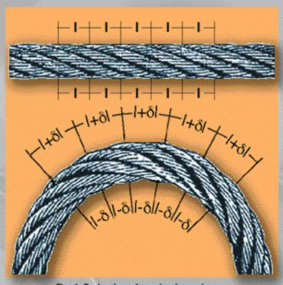
Fig. 4: Reduction of tension in a wire rope
