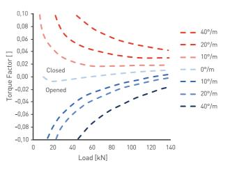
Conversely, a measurable twist for each reference length can again be determined earlier in the case of non-rotation resistant ropes.
