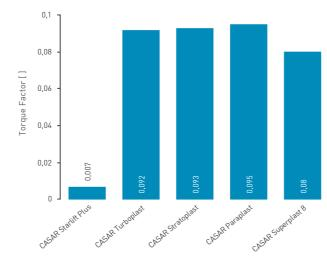
Rotation resistant ropes have a small torque factor, but build up a very high torque resistance when twisted violently. Non-rotation resistant ropes such as the Stratoplast naturally tend to untwist, but are more robust against violent twisting, for example due to larger deflection angles.
