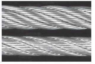
The same rope before swaging (top) and after swaging. Hammered ropes have much greater contact areas with the grooves of sheaves and drums than conventional steel wire ropes with a "rough" surface. This leads to much lower contact pressures and as a consequence to much lower sheave, drum and rope wear.
