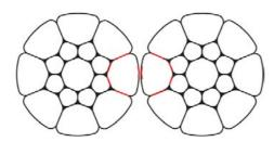
While conventional strands are designed with a fill factor up to 0.82 (or 82% amount of steel in the strand, depending on the strand design, e.g. Seale, Warrington Seale, etc.), the strand compaction can achieve fill factors of 0.90 and
