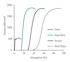
The actual elastic expansion is reversible and proportional to the load. A rope with a high E-modulus tends to be stiff, whereas a rope with a low E-modulus tends to have a high energy absorption capacity and is correspondingly less sensitive to shock loads.
