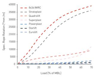
Rotation resistant ropes only show measurable twisting significantly above the loads that occur in use.
