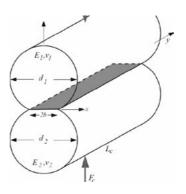
Figure 8: Cylinders in contact
