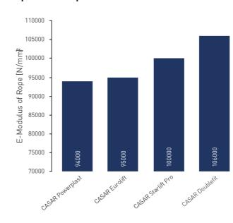
The realistic figures are depending on many influences, most important the type of rope and rope design, the range of loads as well as the number and frequency of loading cycles of operation.
