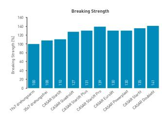
The breaking forces and the fill factors of the CASAR special wire ropes are significantly higher than the breaking forces of the standard designs (DIN EN 12385-4).
