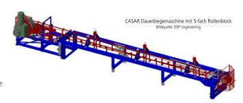
Following diagrams show the service life values determined in the laboratory on a permanent bending machine with the same relative loads and with the same diameter ratio (D / d = 20) for the non-rotation resistant CASAR ropes as well as the rotation resistant CASAR ropes.
