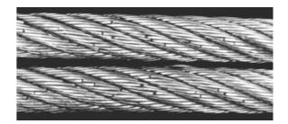
Fatigue cracks in a steel wire rope
