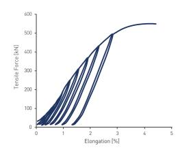
Load/Strain diagram for a wire rope
