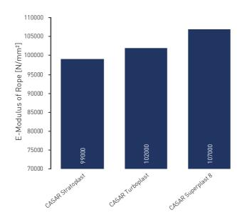
The values for the E-modulus of the ropes are about half as high as the value of steel. The values given in the diagram are average values from a large number of tests with different diameters.
