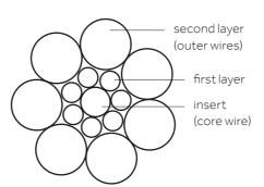
Properties like fatigue resistance and resistance to abrasion are directly affected by the design of strands. In most strands with two or more layers of wires, inner layers support outer layers in such a manner that all wires may slide and adjust freely when the rope bends.
