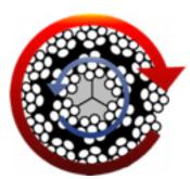
With such a high residual moment, significant rotation can be expected, even though the rope is classified as a rotation resistant rope. The use of these rotation-resistant or "non-spin" wire ropes, constructed with more than one layer of strands, wound in opposite directions, is the common practice on friction winders around the globe, serving deeper depth of wind shafts.
