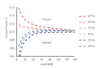
The torque factor is only marginally influenced by the twist. In contrast to this, the torque factor of a rotation resistant rope is significantly influenced by an external twist.
