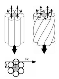
The helically formed strands of a wire rope under tensile load, tend to unwind. Therefore a rope specimen under tensile load with its two ends restricted from rotating, relative to each another, develops torque. The torque induced is a function of the tensile load applied to the rope and the relative rotation introduced between the two ends of the specimen, before the application of the tensile load
